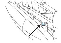
6. HORIZONTAL AIM IS NOT REQUIRED FOR THIS VEHICLE AND IS NON-ADJUSTABLE.
